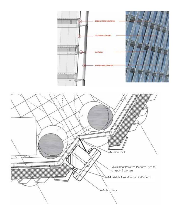
designed to provide safe and efficient access for glass replacement. Introducing the catwalk as one of the major façade elements contributes toward the increase of the cleaning cycle frequency from 4 times per annum to 15 times per annum, which is calculated with three BMU's on the roof with capacity for three workers per platform.
