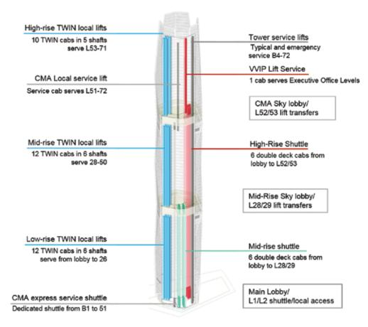
Opposite: Elevator system configuration showing use of double deck and TWIN cabs. Source: HOK
